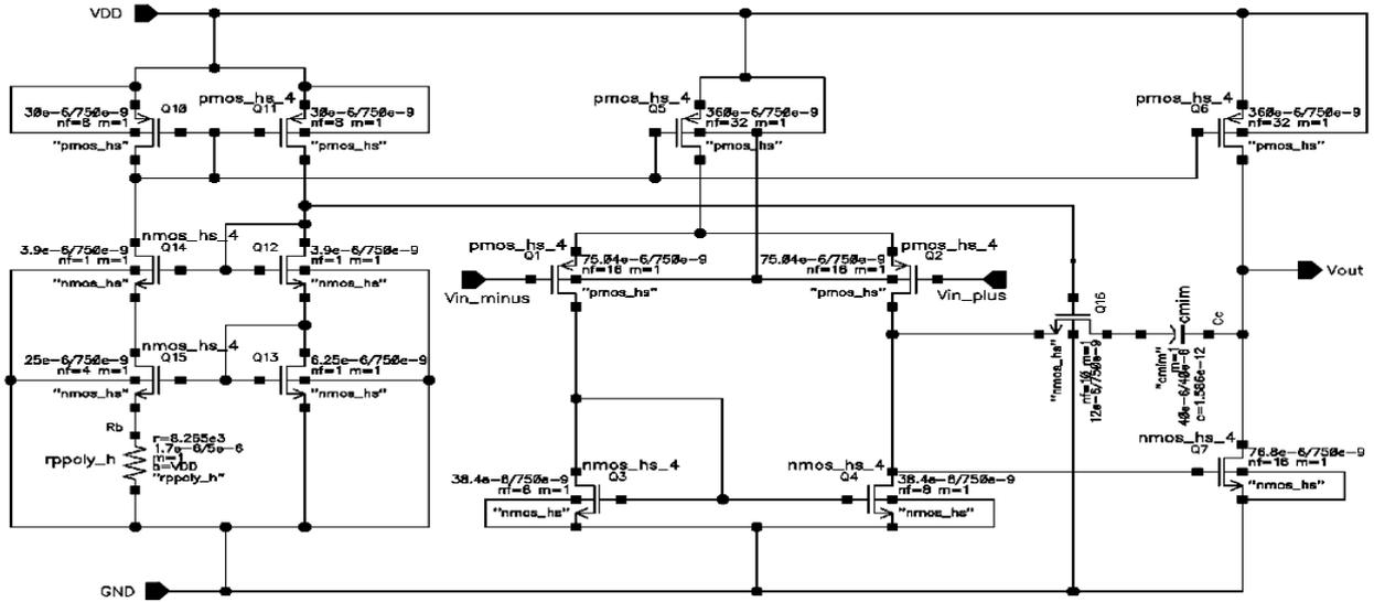
Fig. 1. Schematic of the two-stage op amp circuit.
