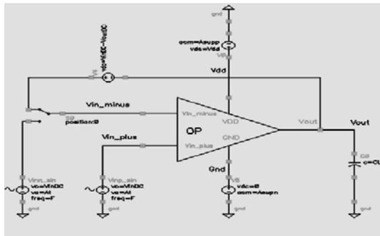
Fig. 2. Test bench circuit for the op amp.
