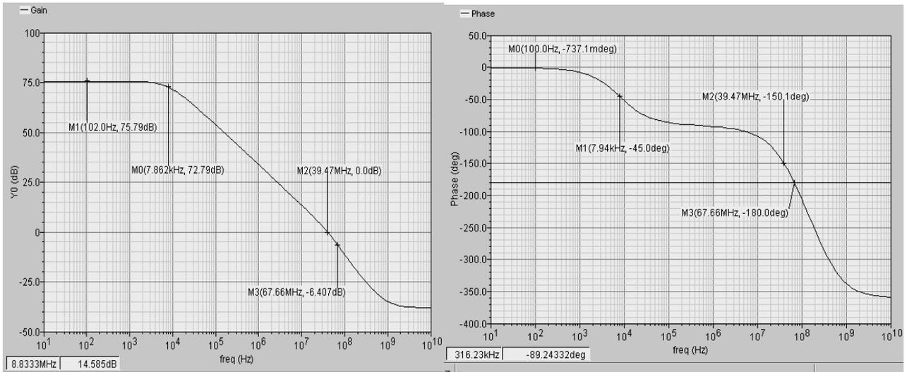
Fig. 4. Simulated transfer function of the op amp with just the Miller's capacitor  $C_C = 1.586$  pF.
